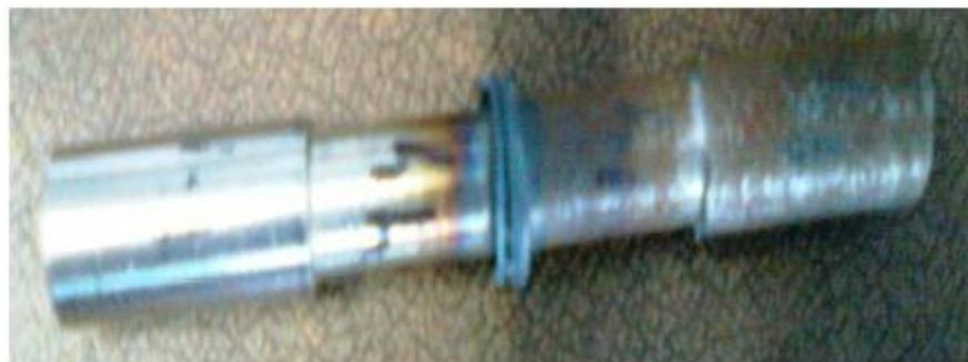
**Figure 1: Micrograph of friction welded specimen**
