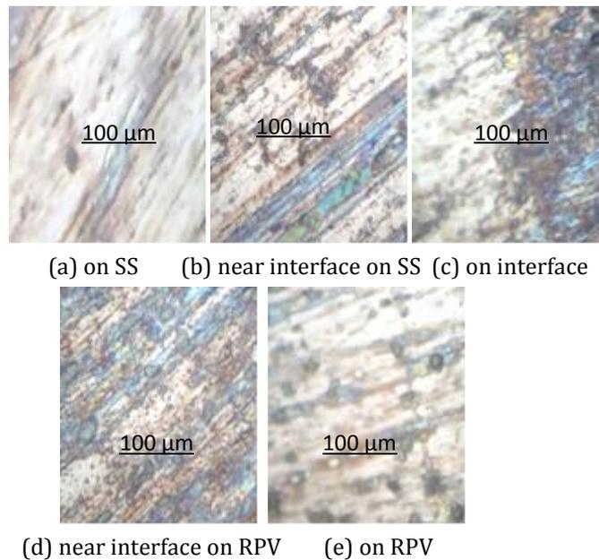
**Figure 2: Micrographs on different zones of the welded specimen**
