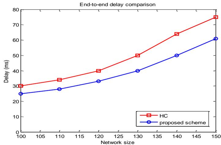
**Figure 5: End-to-End Delay Comparison between Classic Hop-Count Routing and Proposed Routing Scheme**
