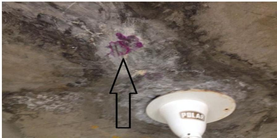
Figure 4: Pink colour after spraying of phenolphthalein
