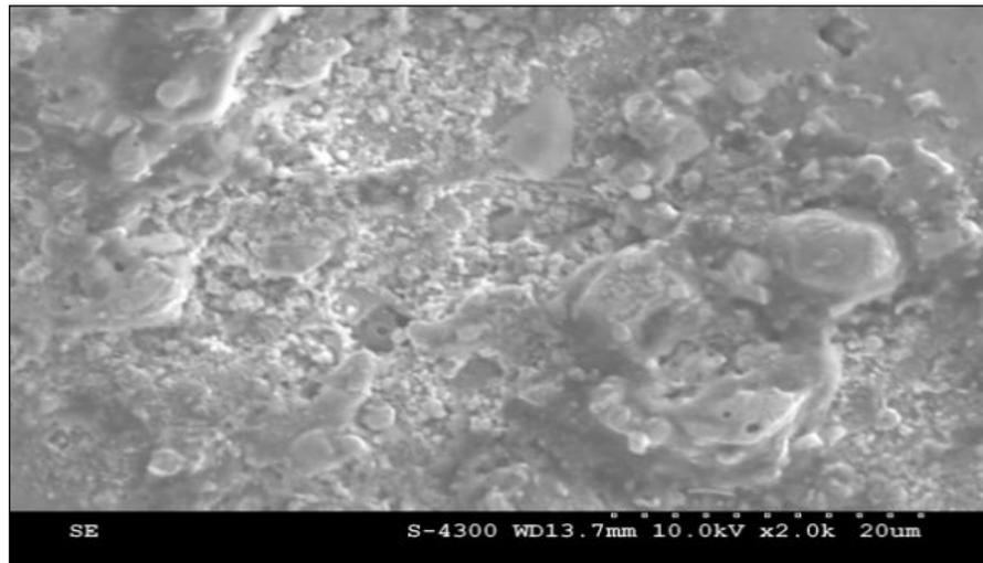
**Figure 6: SEM micrograph at 2000× of Al 6061 machined with green compact copper electrode (I 9Amp, pulse on time 100μs)**
