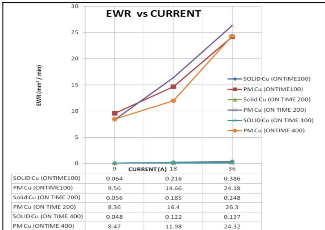
Figure 3: EWR vs Current for Solid and PM Cu Electrode at different Pulse On-time
