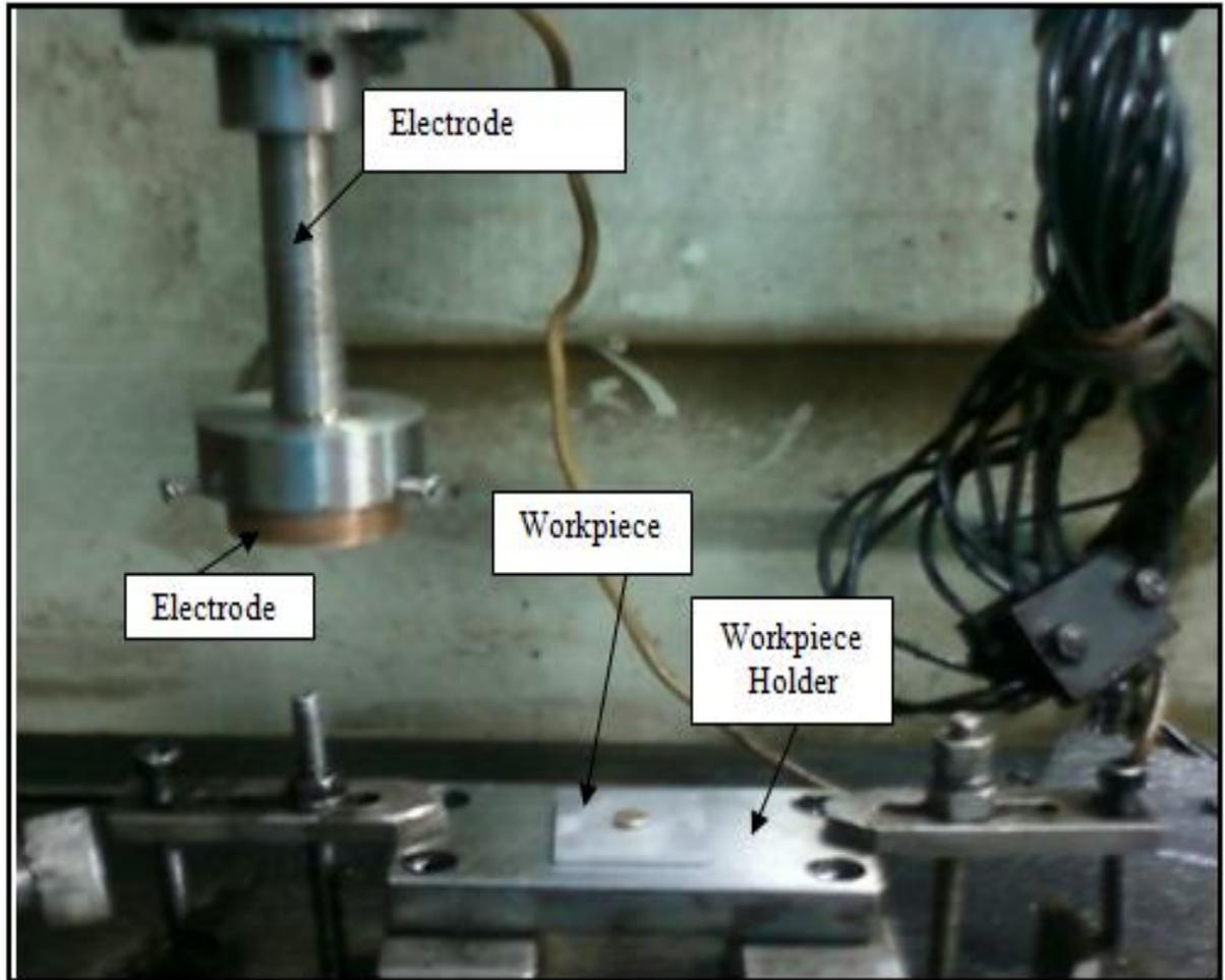
**Figure 1: View of the experimental set-up of EDM machine**
