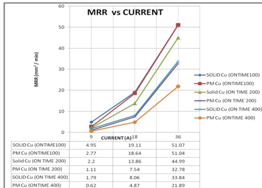
**Figure 2: MRR vs Current for Solid and PM Cu Electrode at different Pulse ON Time**
