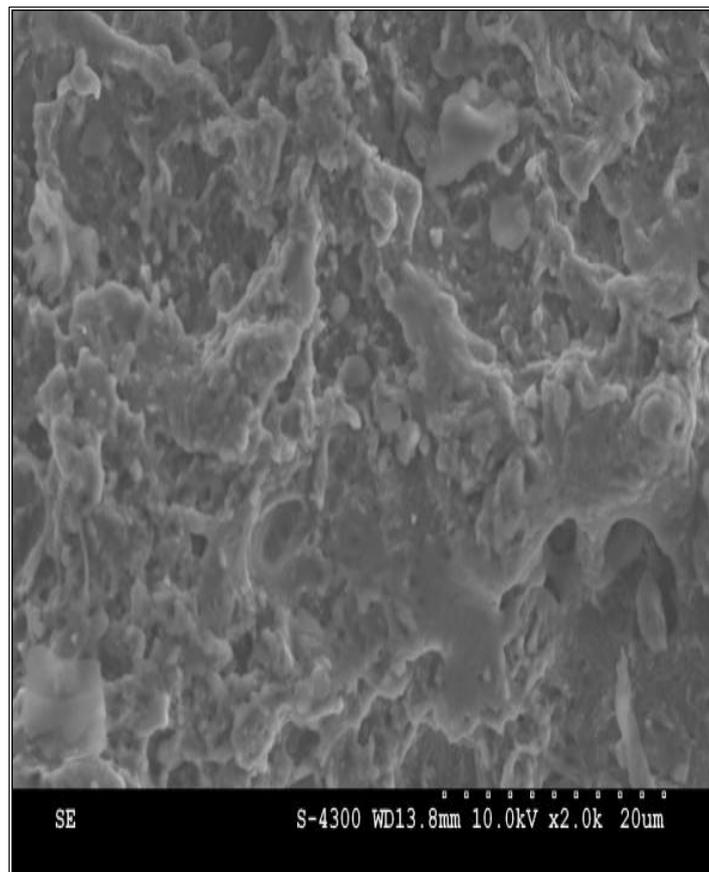
**Figure 5: SEM micrograph at 2000× of Al 6061 machined with solid copper electrode (I 9Amp, pulse on time 100µs)**
