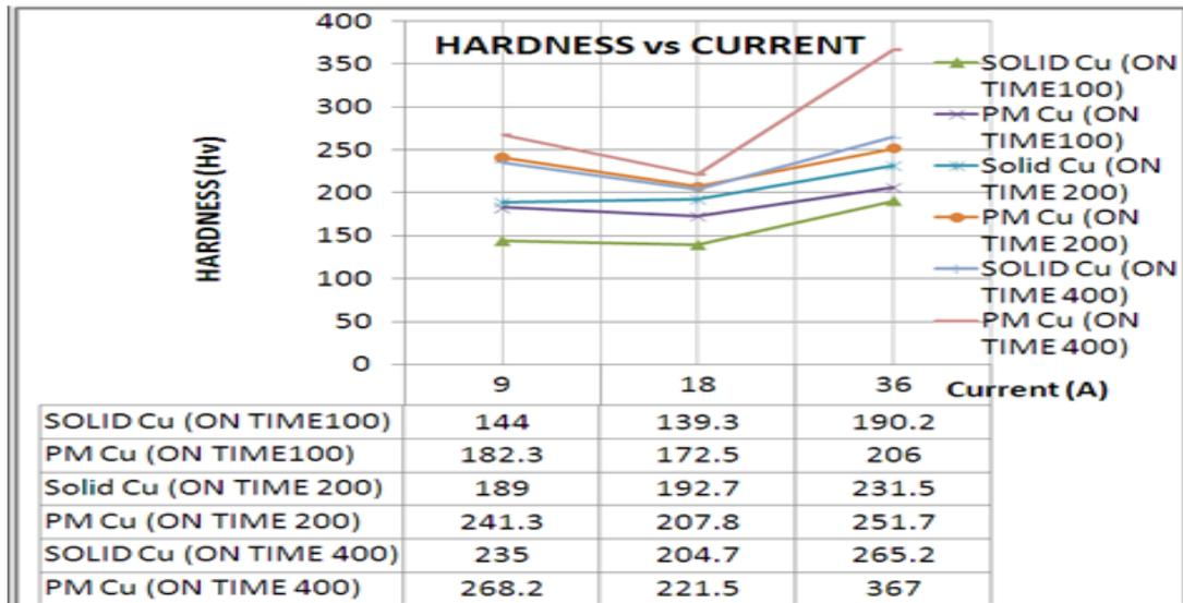
Figure 4: Hardness (Hv) vs Current for Solid and PM Copper Electrode at different Pulse On-time
