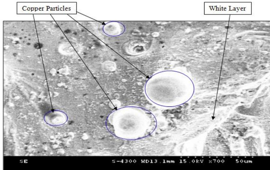
Figure 7: SEM micrograph at 700× of Al 6061 machined with green compact copper electrode (I 36 Amp, pulse on time 400µs)
